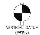
NAVD 88 ESTABLISHED USING GPS RTK ROVER CONSTRAINED TO THE WASHINGTON STATE REFERENCE NETWORK (WSRN) STATIONS
