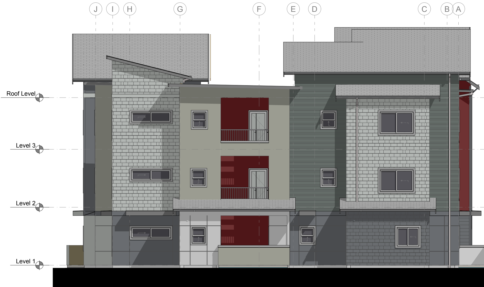
2 RIGHT ELEVATION -BUILDING TYPE No. 1 SCALE: 1/8" = 1'-0"
