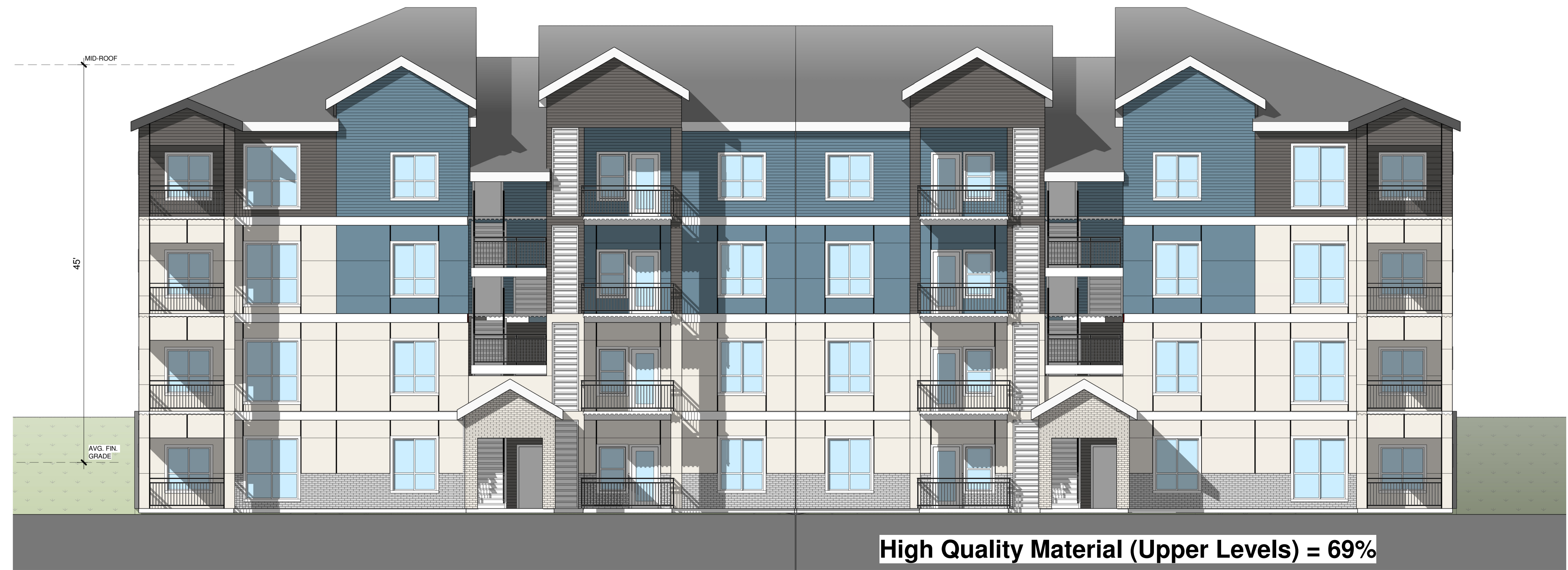
Building K - North Elevation / 27th Ave SE . 1/8" = 1'-0"
