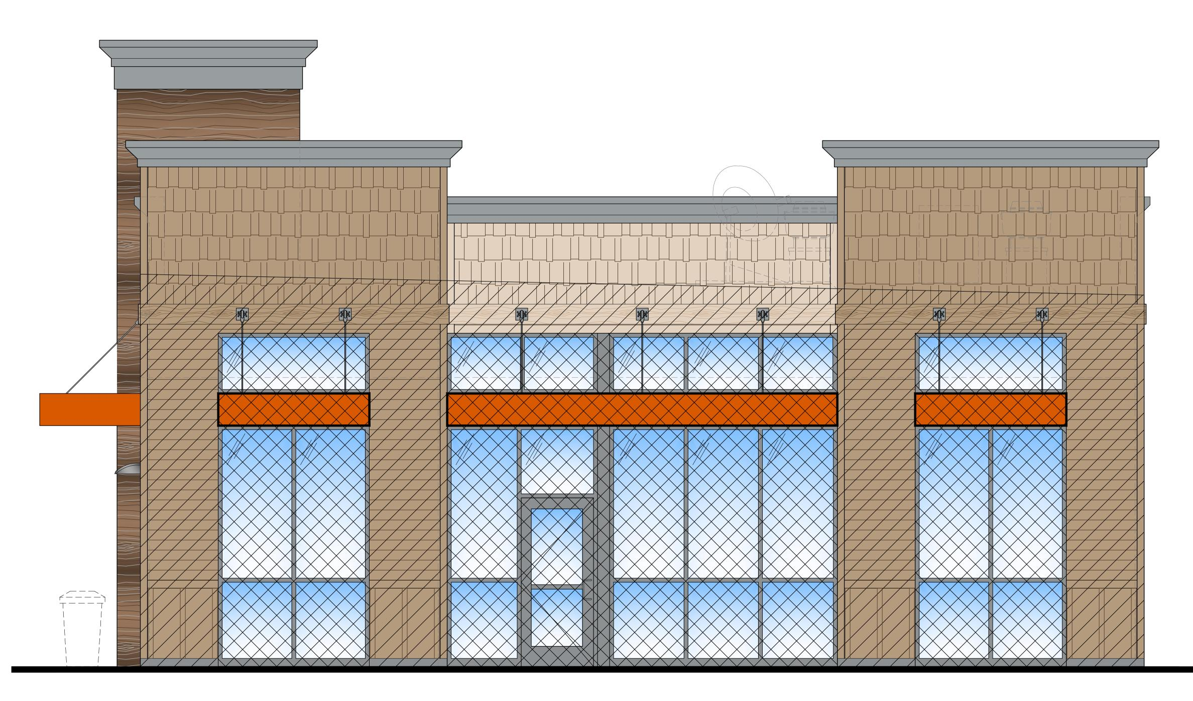
TOTAL AREA FROM FINISH FLOOR TO TOP OF ROOF = 660 SF MINIMUM TRANSPARET AREA: PROPOSED TRANSPARENT AREA: 397 SF; COMPLIANT
