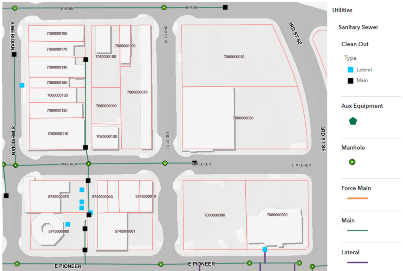
Figure 5. Existing Sewer Infrastructure On and Adjacent to the Cornforth-Campbell Properties
